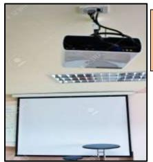
LCD projectors are used when output is required on a big screen. Instead of on a monitor, the output is projected on the big white screen through the LCD projector.
